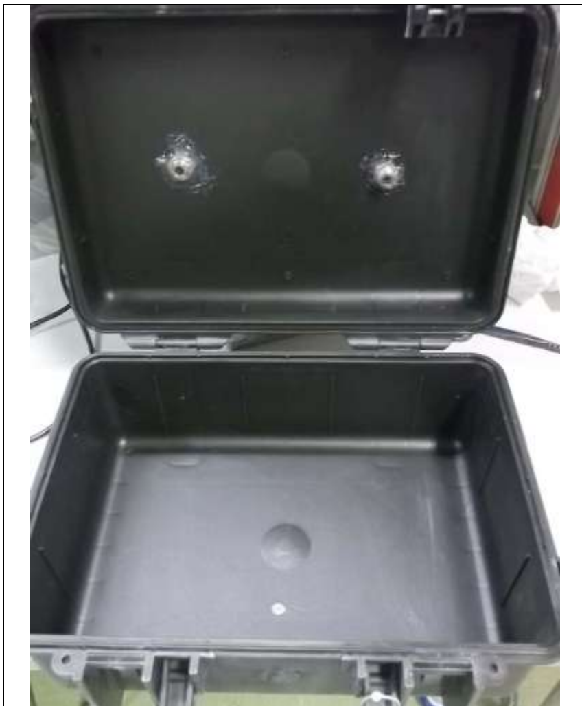
Photo 3: Result of the test to verify the protection degree IP 6X
