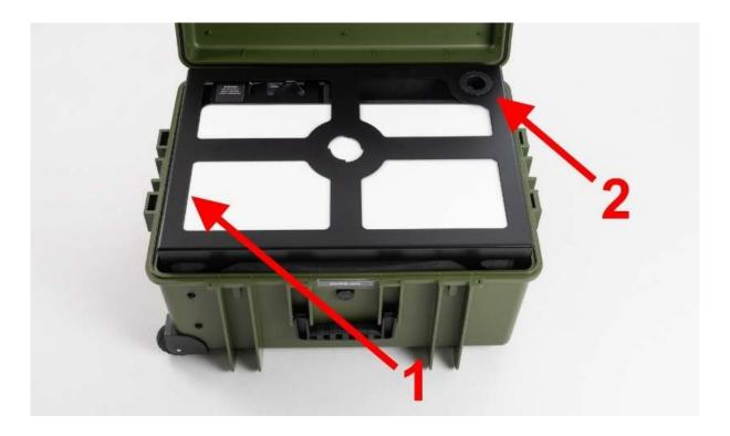
One side of the cable can then be plugged into the Starlink aerial from below. Caution! Make sure that no dirt gets into the plug connection! Particular care must be taken here! The aerial can then be plugged into the aerial holder (1) as shown in the following illustration. Ensure that it clicks into place and is correctly orientated in the antenna holder.
