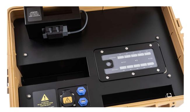
If an RJ45 module has been ordered, the next step is to insert the RJ45 into the holder and connect the cable of the RJ45 module to the Starlink router and stow it away properly. The two illustrations below show where the plug of the RJ45 module is inserted into the Starlink router and how the connection cable of the RJ45 module is best stowed away.
