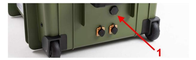
The cable with the pre-installed sleeve must then be fed through the now open side hole from the outside. The correct positioning can be seen in the following illustration. From the inside, the plastic nut is guided over the plug of the cable and over the cable up to the thread of the sleeve, fitted and screwed on hand-tight.
