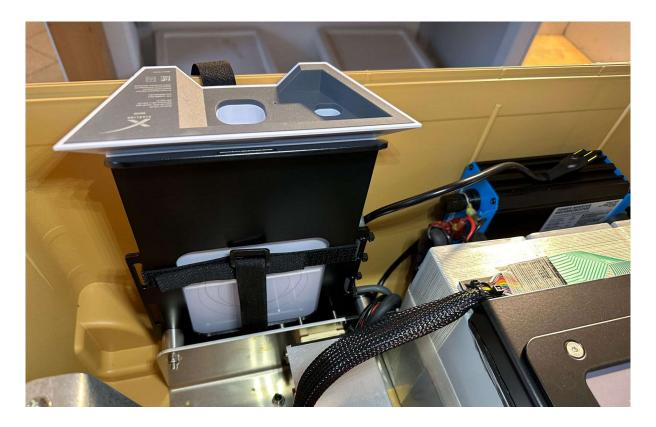
Then plug the pre-installed power cable firmly into the Starlink router and secure the plugged-in cable with the horizontal Velcro strap. Special care must be taken to ensure that the Velcro strap runs over the inserted cable and is carefully tightened. The following illustrations show the procedure and the exact position of the Velcro straps after installation.
