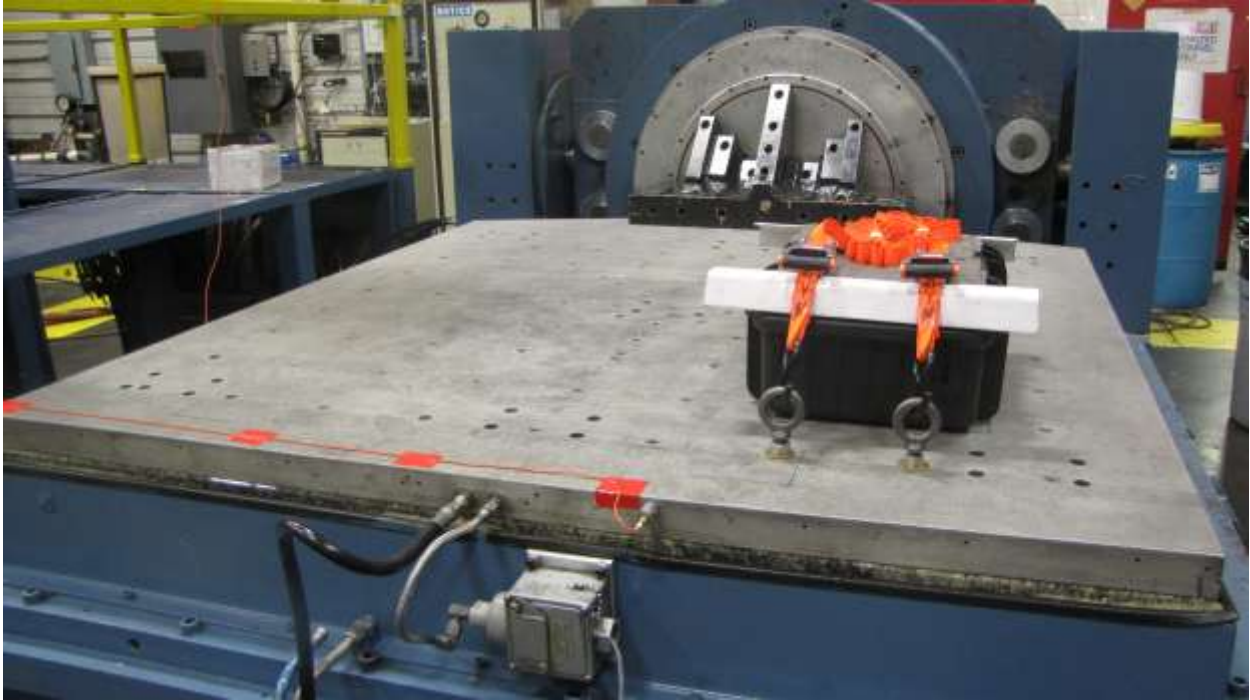
Photograph No. 5 Typical Sinusoidal Vibration Test (K) Setup (Side-to-Side Axis)
