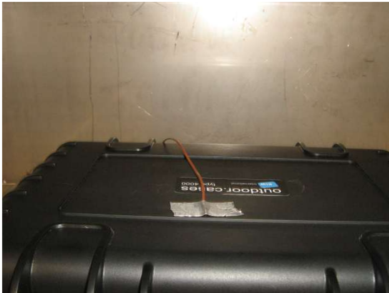
Photograph No. 2 Typical Low Temperature/Dry Heat Test Setup (Thermocouple Location)
