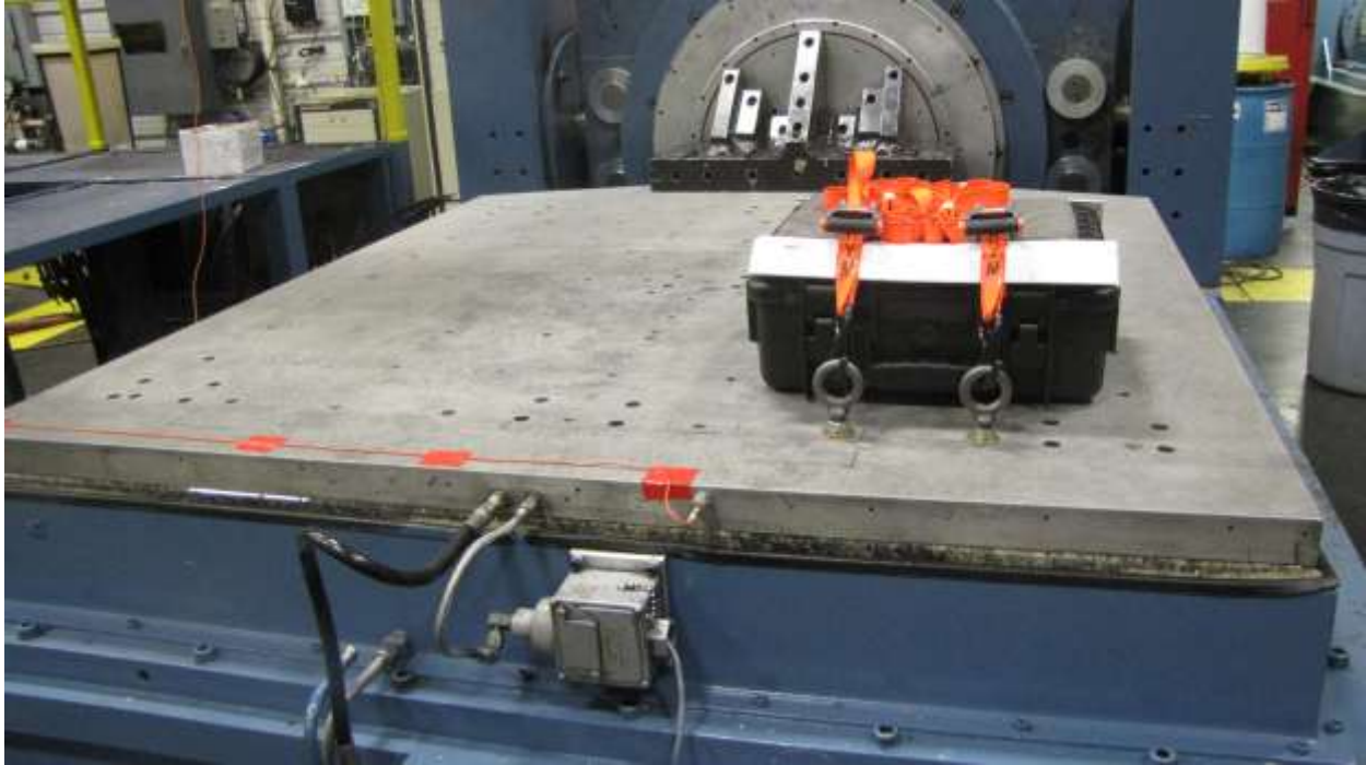
Photograph No. 4 Typical Sinusoidal Vibration Test (K) Setup (Front-to-Back Axis)
