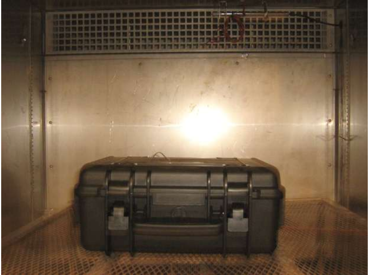
Photograph No. 1 Typical Low Temperature/Dry Heat Test Setup
